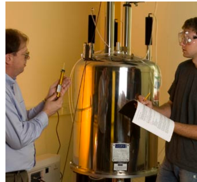
Dr. Lance Whaley (left), assistant professor of chemistry, uses the nuclear magnetic resonance (NMR) spectrometer in many of his research endeavors. The NMR spectrometer is useful in determining the structures of molecules.
