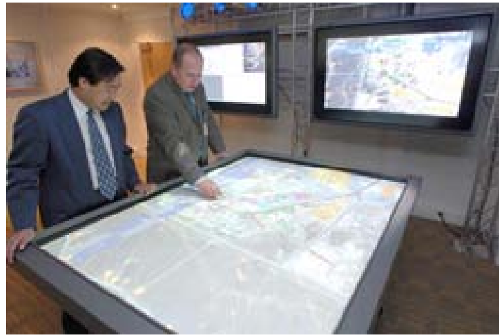
The TouchTable® is a geospatial environment for manipulating data that enables images and live GPS tracks to be used together in a collaborative headquarters setting.
